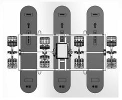
Stakes should be placed as straight up and down as possible so the paddle wheel is able to rise and fall with changing water levels. If extra staking is needed, do not use stakes with a rough surface that could catch the metal loops of the frame and prevent the water level adjustment
