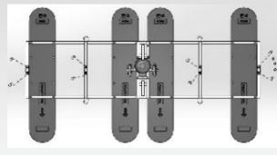
Before moving on to the next step, examine the paddle wheel axles. Several notches are taken out of the axle for securing the paddles to the axle and connecting the axle to the couplers. The notches are not numbered on the axle itself, but for illustration they are numbered as shown below. The notches are numbered from the inside of the paddle wheel out
