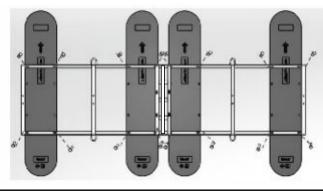
On each long side of the frame, measure from the outer edge of the frame to the first hole encountered on the centre crossbars. On one side the hole will be approximately 22" from the edge, and on the other side the hole will be approximately 19" from the edge. The short side (22") should be on the same end as the water flow as indicated by the floats.
