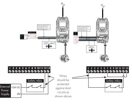
NOTE The Maximum cable length from Voltage source to the drive terminals should not exceed 25 mtrs.
