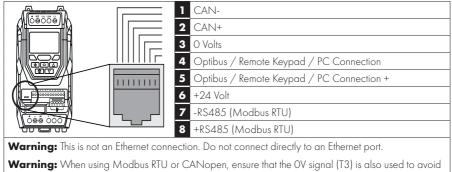
comms errors and potentially damaging common mode voltages.
